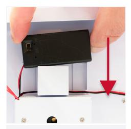
5. Slide down the battery pack into the holder.
