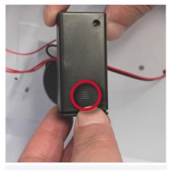
3. Remove the battery pack cover by sliding it upwards.
