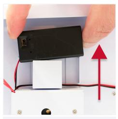
2. Slide the battery pack upwards from the holder.
