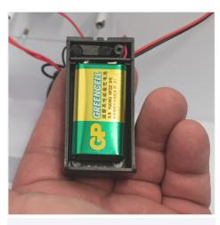
4. Insert the battery and replace the battery pack cover.
